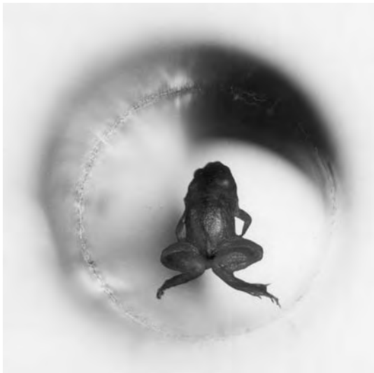
Figure 6.8 A small frog floating above a high field superconducting magnet, due to diamagnetic repulsion. (Photograph courtesy of A. Geim, University of Manchester.)
